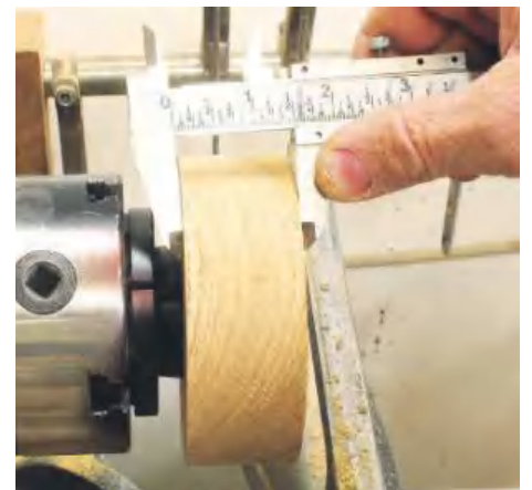
▲ Pic.9 To achieve good copies the sticks will need to be the same height. Measure the thickness of the base so that measurement can be transferred to the other one(s)
